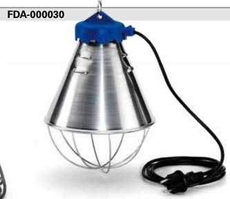
Aluminium reflector Ø 210 mm, complete with mt 2 chain, protection grid, mt 2,5 cable schuko plug spray proof, heavy porcelain  $\varnothing$  54 screwed lamp holder, maximum power: 250 W
