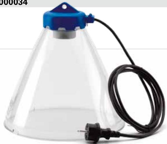
Transparent polycarbonate reflector Ø 270 mm, heat resistant, unbreakable, mt 2,5 cable schuko plug spray proof, heavy porcelain Ø 54 screwed lamp holder, maximum power: 250 W
