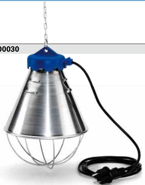
Aluminium reflector Ø 210 mm, complete with mt 2 chain, protection grid, mt 2,5 cable schuko plug spray proof, heavy porcelain Ø 54 screwed lamp holder, maximum power: 250 W
